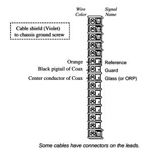
Figure 7-7 Terminal Designations for Direct pH/ORP with Quick Disconnect Option
